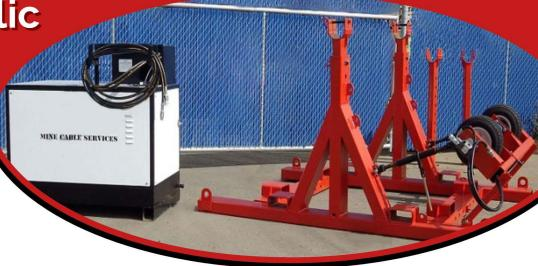
Mine Cable Services has designed and manufactured its Rim Drive Cable Reeling system for versatility and ease of use. Featuring a fully adjustable frame, the MCS Rim Drive Cable Reeler accommodates cable reels from 60"-120" diameter and 48" to 84" wide with a maximum payload of 35,000 pounds (reel and cable). Engineer certified spindles and spacer collars are provided to accommodate the width, weight, and arbor size of cable reels in use at your operation.
